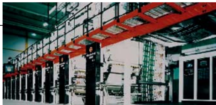
Rotogravure press for packaging printing (W&H)
