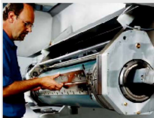
Mounting a flat screen for rotary screen printing
