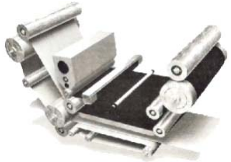
Printing unit based on ionography
