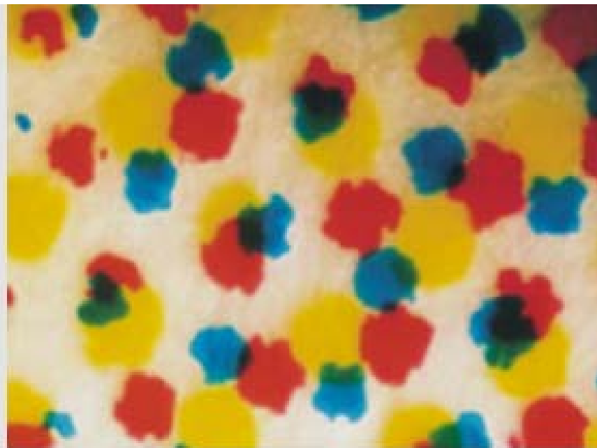
Halftone dots in screen printing Source: H. Kipphan
