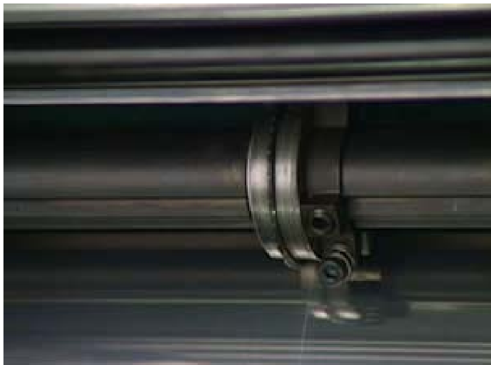
Perforating unit in operation (after printing)
